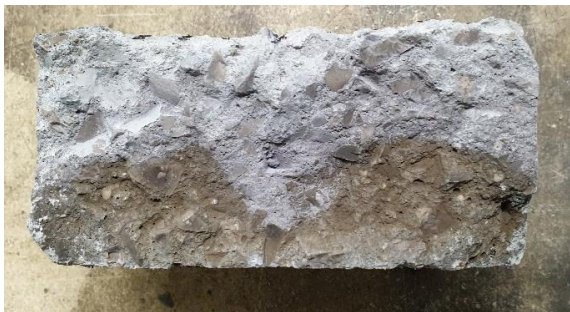
Fig. 8 – Specimens subject to chloride attack
