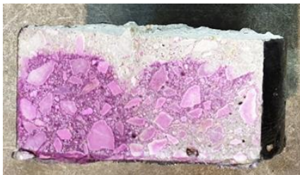
Fig. 4 - Reaction of the phenolphthalein in specimens subject to carbonation test
